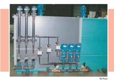
In many cases, the F series Moineau pump can be used as a dosing pump. It is an advantageous replacement for traditional dosing units for highly viscous, articulate or abrasive products.
